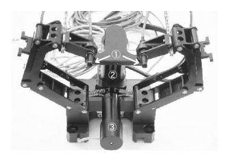
Figure 10. A Prototype of a constant-orientation link:
