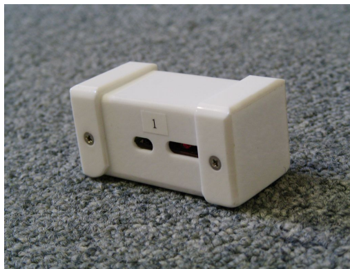
Figure 4: Wireless tactor unit installed in a case.
