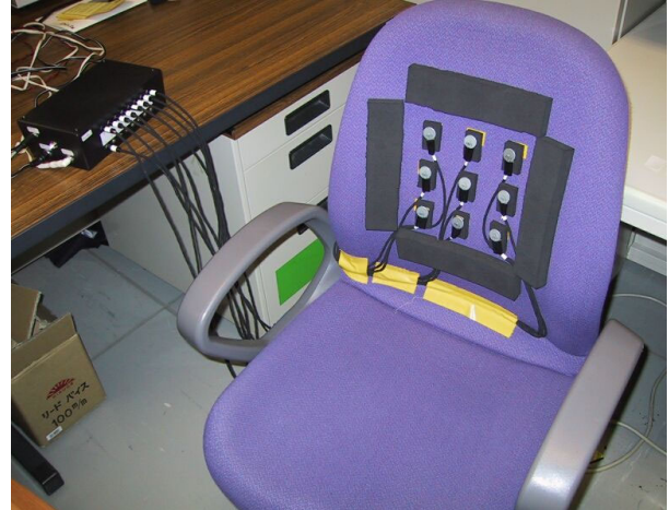
Figure 1. Office chair with 3-by-3 tactor array
