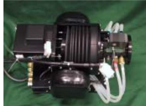
Fig 13: Accordion type air cannon.
