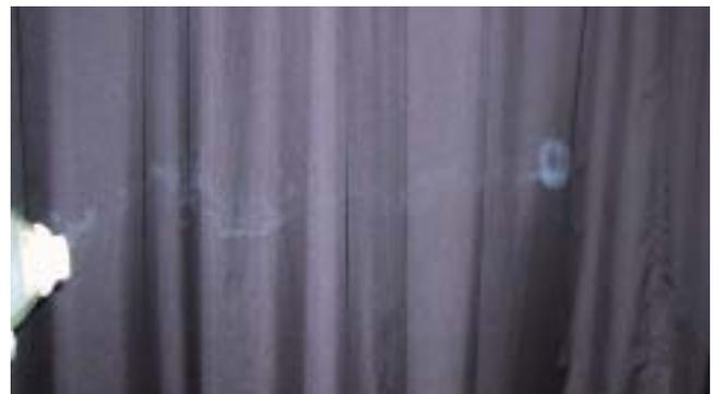
Fig 3: A smoke ring launched from an air cannon.
